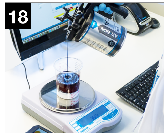
Prepare the mixture for color matching test according to the recalculated recipe. If the end result is satisfying - job is completed. The process can be repeated any number of times.
