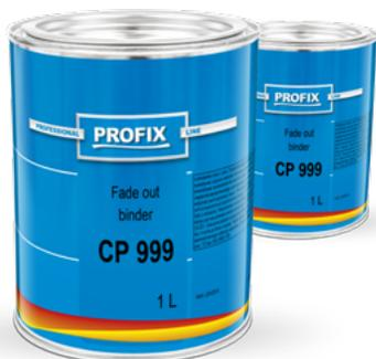
Shading resin is a single-component product used for painting car bodies. It is intended to balance the color difference between the special coat 1K primer and the old coat surface on the surrounding car elements (or on the same element in the case of touch-up paintings).
